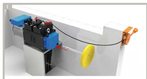
Step 1: put the hand wheel into machine, until the gear of hand wheel and machine completely in mesh.
