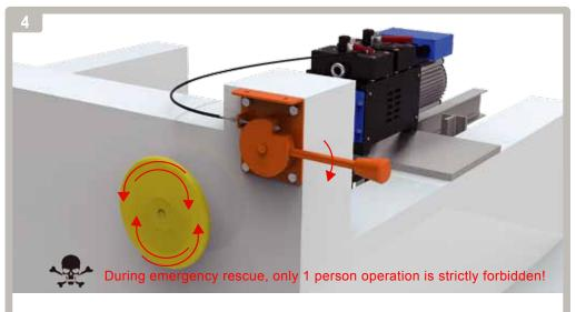
Step 4: In using, put the hand wheel into bushing cover, until the gear of hand wheel and machine completely in mesh. First, hold the hand wheel tightly, another person release the break. Then could clockwise or counter-clockwise the hand whee, I operate the hand wheel to adjust machine.
