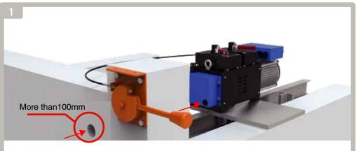
Step 1: after machine installation, make hole on the wall side according to hand wheel install position, the hole on the wall should larger than outer diameter of wall bushing cover(bushing cover dia 42mm).
