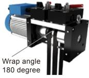
Note: this guide wheel and anti jump bar only apply for the wrap angle within 180 degree!
