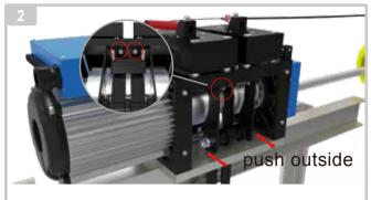
2 Loosen the screw, push outward the guide wheel to the end, if not sufficient space left, no need to do like that.
